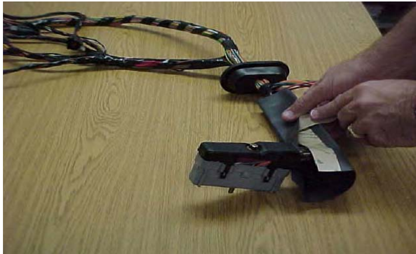
Photo 4 Installing PRT-S around the cable.
