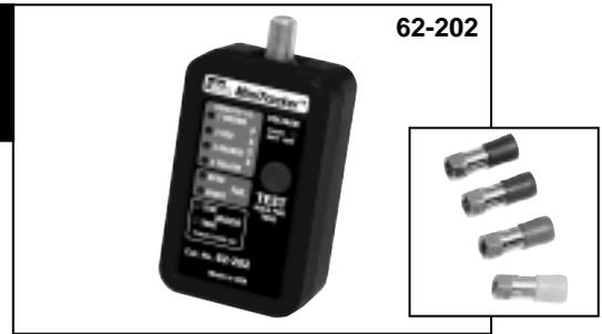
Testing of coaxial cable generally consists of checking for opens or shorts in the cable. Use the **IDEAL MiniTracker Tester** (62-202) to test for opens or shorts in the cables terminated with F-connectors. This tester can be used through a standard splitter or individual runs of cable and also to trace cable for identifying cable runs.
