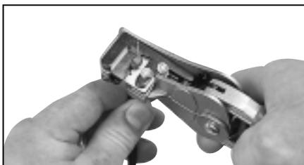
Switch cable into larger stripping hole and strip off approximately 1/4" of outer jacket.
