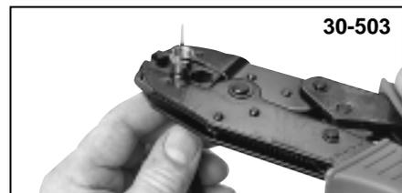
Crimp F-connector using **IDEAL Crimpmaster<sup>™</sup> Crimp Tool** (30-503). Insert cable and connector into appropriate die nest of crimping tool. Center the 3 rings on back of connector in the die of tool. This die crimps RG-59 or RG-6 F-type CATV connectors. Squeeze handles until the crimping tool releases and remove cable and connector.
