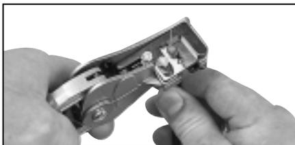
Insert cable into tool as shown and squeeze the handles to strip cable. Strip using small hole first, leaving 1" of center conductor exposed.
