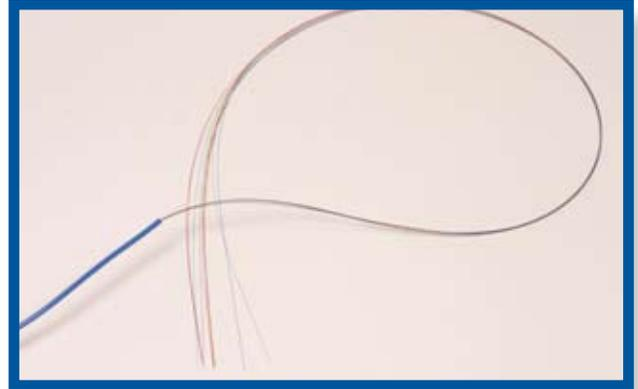
**1.3** Place the fibers in color-coded order in the fiber arrangement tool.
