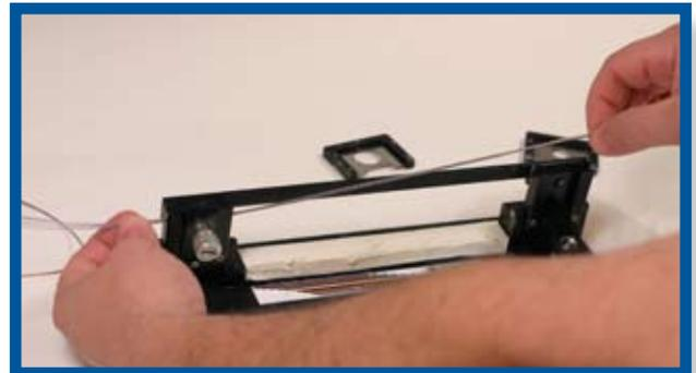
**1.9** Snip the excess fiber ends that are not ribbonized in preparation for splicing.
