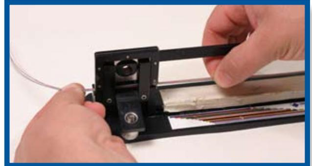
**1.8** Allow glue to dry and remove fiber from holder. While holding the ribbon, unhook the bracket(s) and slowly lift up the ribbon.
