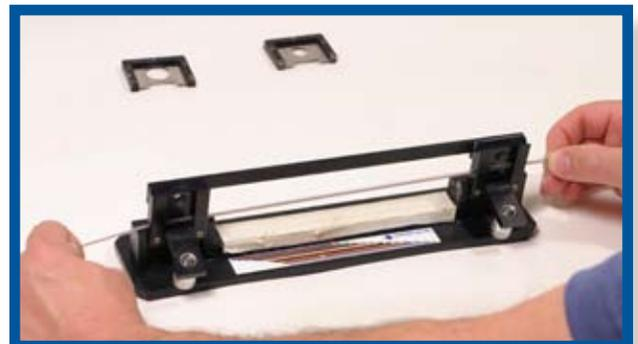
**1.6** While maintaining gentle pressure on the fiber ends tighten the fiber clamps.
