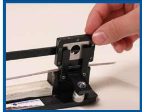
**1.5** Grasp the fibers and pull them back, aligning the fiber ends within a 1/2-inch of the tool's edge.
