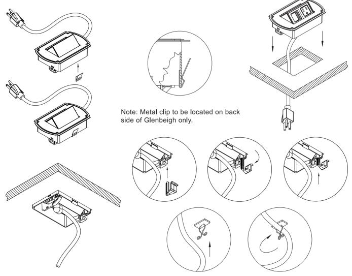
Note: In a conduit application; conduit should be supported according to local code.
