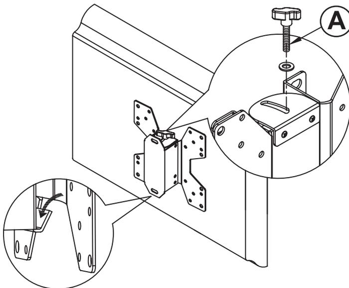
**Figure 6 - Attach TV Assembly to Wall Plate**
