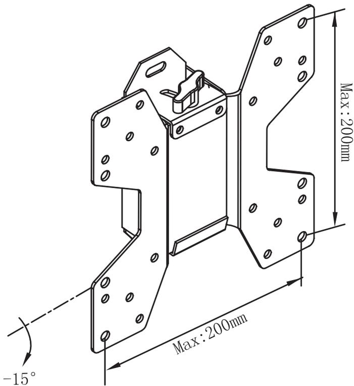
**Figure 7 - Adjust Angle**
