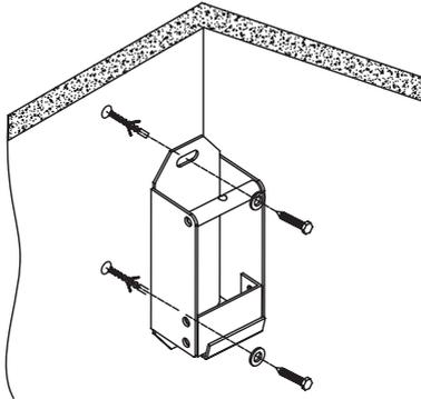
**Figure 3 - Wood Stud/Concrete Mounting**
