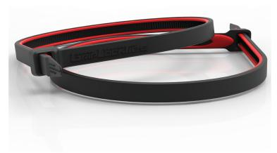
The unique rubber lining of GripLockTies™ eliminates the tendancy to over-tighten and distributes the tension more evenly around a wire bundle, eliminating damage to wires at a single friction point. The releasable tab allows you to remove or reset your tie, even after snugging it tight, saving you from wasting ties when running multiple wires or when you forget that last wire.
