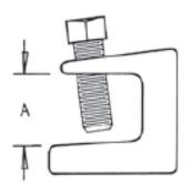
Malleable Iron-Plated Beam Clamp
