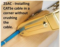
Model 25AC IS designed to drive the specially configured staples to a pre-determined depth in most substrates, thus making it virtually impossible for the Broadband wires to be crushed. (US Patent no. 6,848,607)
