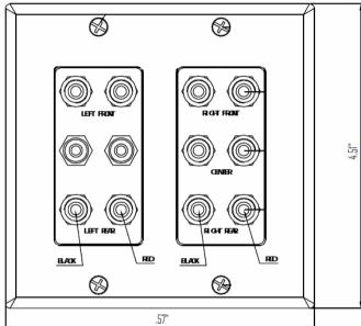
Installs in a NEMA 2-gang box or low-voltage mounting bracket.
